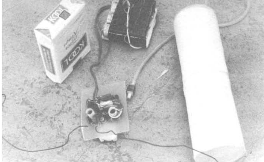
Complete Thermal Sensor system from Hill's glider. Transmitter and audio circuits are on small board at left center. Sensor is just to right of circuit board. Batteries (4 Nicads) and an air bottle made from two foam coffee cups are also shown. A dipole antenna is used for efficiency. This is taped to wing along leading or trailing edge.
